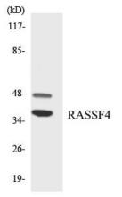
Western blot analysis of the lysates from RAW264.7cells using RASSF4 antibody.
